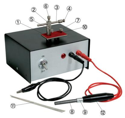
Use crocodile clip on black cable to make an earth or negative connection by clipping on to base ①. The other end has to be inserted into the black plug on apparatus. Use the red cable to make a positive connection by inserting the end into the red plug on the apparatus. The other end has the carbon stick ⑨ for soldering.
